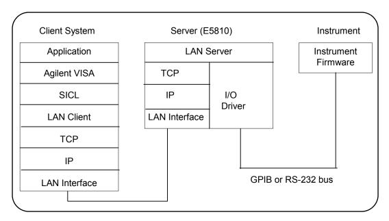
How IO Application Software Works With the E5810 Before trying to perform an I/O application operation on the E5810 GPIB interface and the GPIB bus, the Remote IO Client software in the client computer system establishes a network connection to the remote I/O server (the E5810). Once the client establishes a connection, the client can begin to send I/O requests to the E5810.
