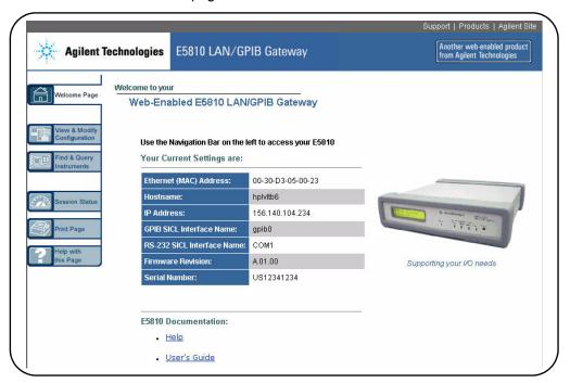
You can use the Web access to configure the E5810 and to communicate with GPIB and/or RS-232 instruments. For example, using the **Configuring your E5810 LAN/GPIB Gateway** page of the E5810 interface, you can view and modify the configuration of the E5810. Or, you can communicate with installed GPIB and/or RS-232 instruments using the **Find and Control Instruments Connected to your E5810** page of the interface. See Chapter 3, "Using E5810A Web Access" for information on E5810 Web access.
