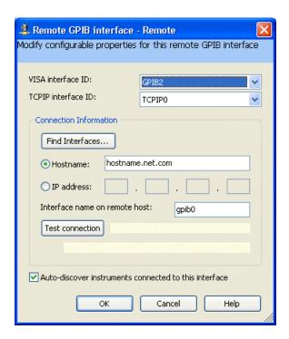
4 Specify the TCPIP interface that you wish to use to host this remote interface, in the **TCPIP interface ID**: field. This must be an interface that is already configured on your system; by default, a LAN interface
