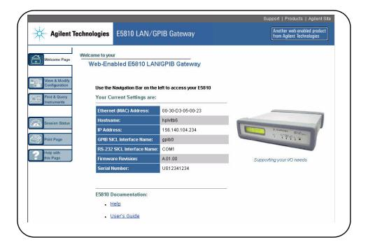
2 Display the Current Configuration Page. from the Welcome page, click the View & Modify Configuration icon to display the Current Configuration of E5810 LAN/GPIB Gateway page
